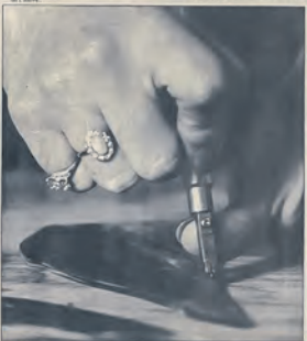
The skilled hands of Frankie Cartner cut a piece of glass to fit a pattern.
